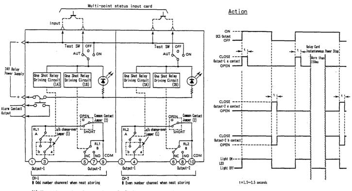
(1) When shipment from factory, Output-1 a/b change-over jumper is in a contact point (2) When shipment from factory, common connect jumper is in connecting status
